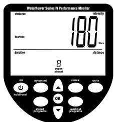
This program allows you to input the volume of water in the tank. The tank volume is necessary in calculation of power (watts).
